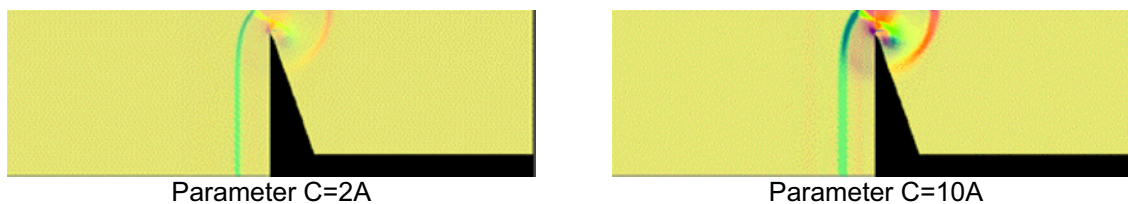
Fig. 5. The CFI-color- schlieren images of the shock wave around the knife-edge flow field (A is a constant).
